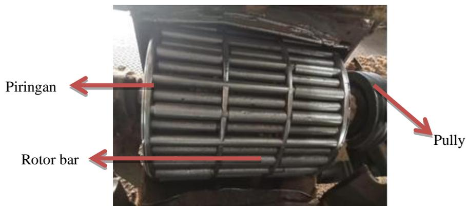
**Gambar. 2** Rotor Bar
