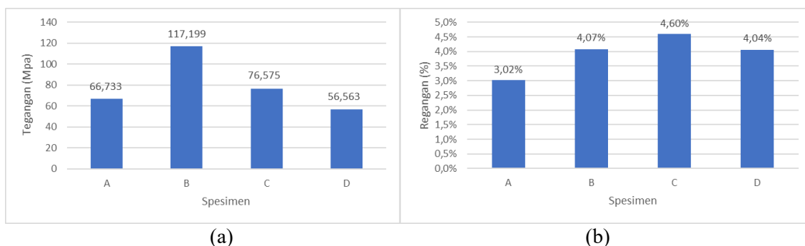
Gambar 4 (a) Hasil rata-rata tegangan tarik (b) Hasil rata-rata regangan tarik
