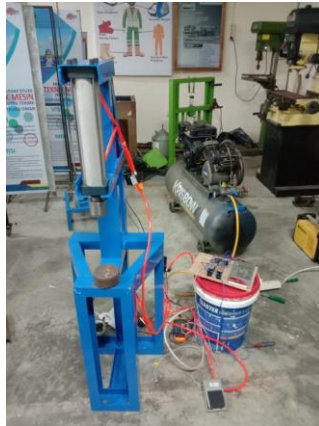
Gambar 3.2 Mesin Pneumatik Power Forging Hammer (Sumber: Penelitian 2021)
