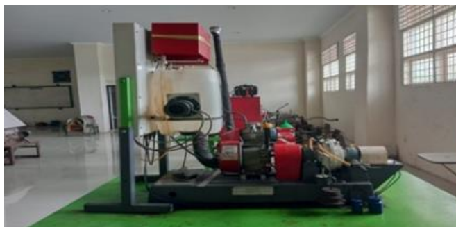
Gambar 1 Mesin bensin Tecquipment TD 115 MKII
