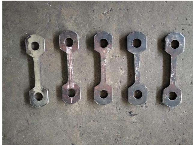
**Gambar 3.** Material benda uji
