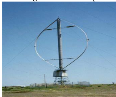
Gambar 7: Turbin angin tipe Darrieus
