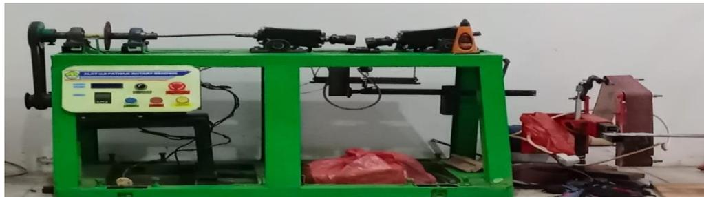
**Gambar 5.** Rotary Bending Machine
