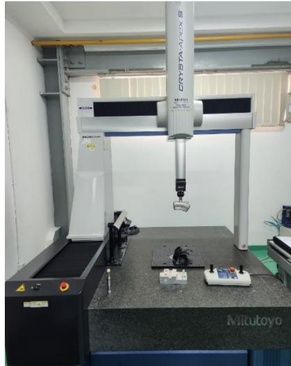
Gambar 3. CMM Type Crysta - Apex S
