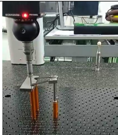
Gambar 8. Proses Pengukuran Gauge Block
