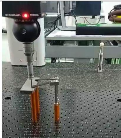
Gambar 8. Proses Pengukuran Gauge Block
