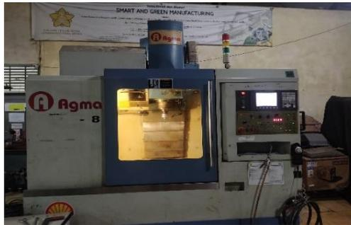
Gambar 1. CNC *Milling* Agma A-8
