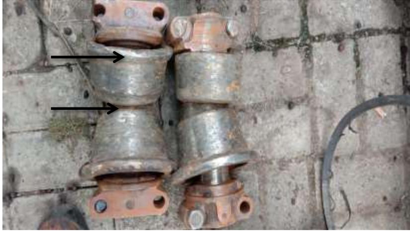
Gambar 2. Track Roller Mengalami Keausan
