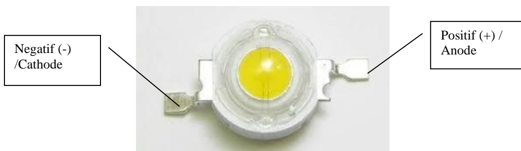
Gambar 3 Diagram elektronik lampu LED. Sumber : http://indoled.host56.com/1_8
