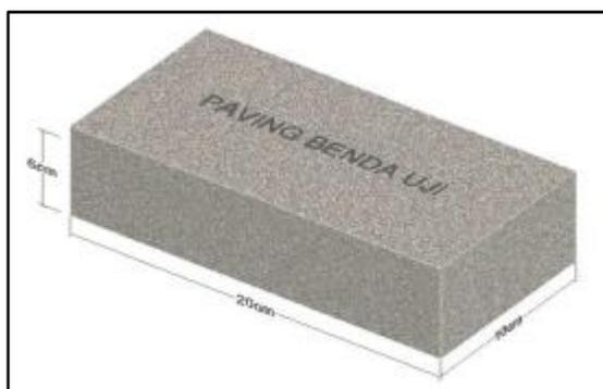
**Gambar 1. Ukuran Benda Uji *Paving block***
