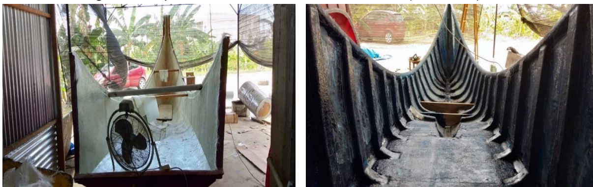
Gambar 3. Gambaran manufaktur Hibrid Material Boat 2 GT
